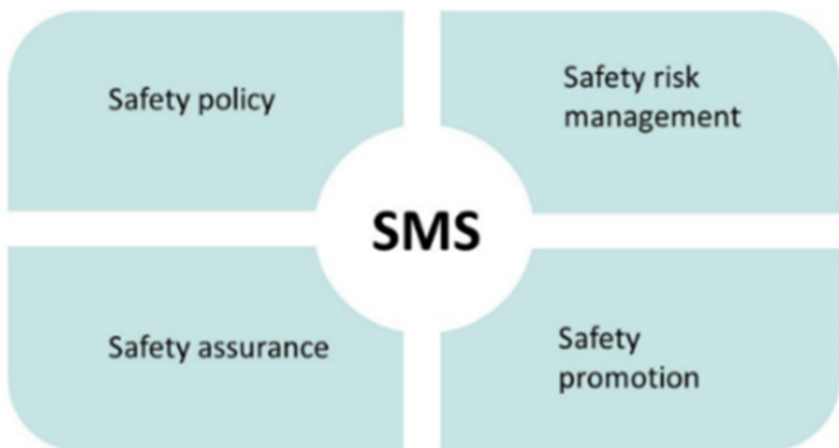
Figure 1 Elements of a safety management system
