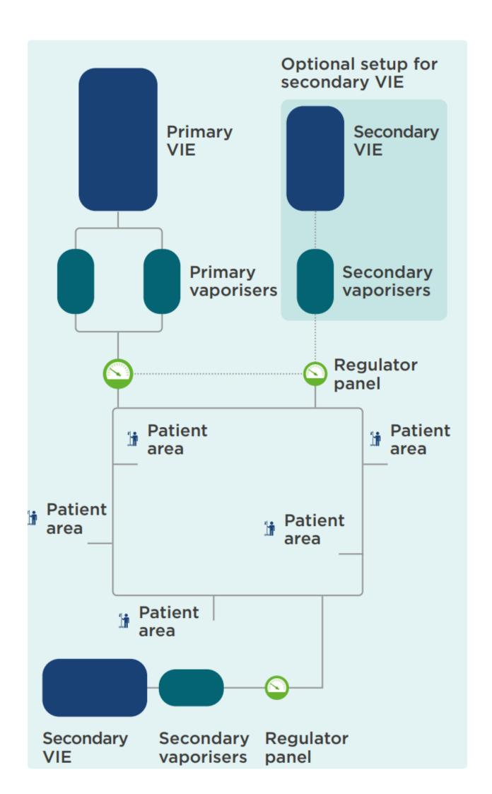
A ring main (Figure 2): a pipeline system which begins and ends at the piped oxygen source so that every outlet has two possible routes of oxygen supply.
