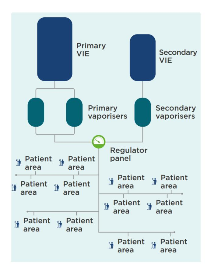
A radial system (Figure 1): a pipeline system which begins at the piped oxygen source and ends at another point so that every outlet has only one possible route of oxygen supply.
